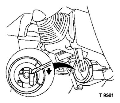
Turn ignition switch to align recess (1) to be opposite lug (2), connect harness plug to switch contact part and insert into steering column lock and fasten with set screws.
