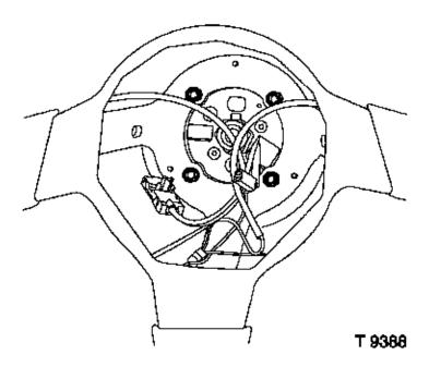
Steering column upper and lower shrouds – screws.
